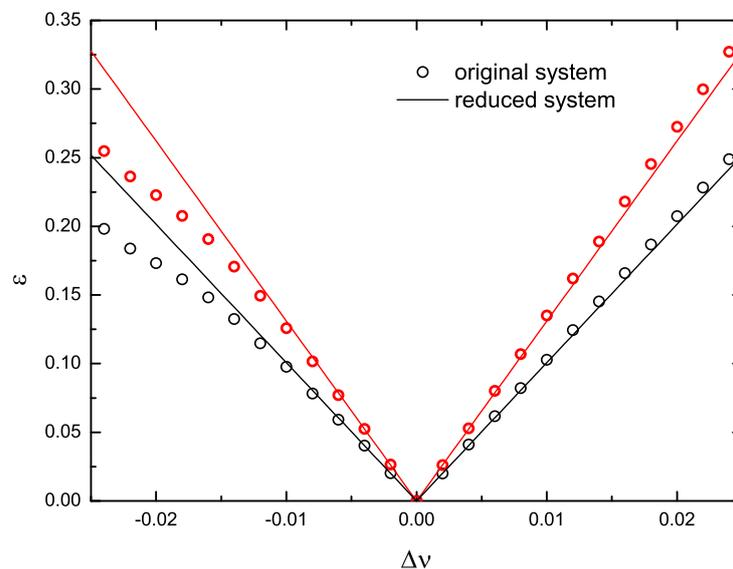
Figure 1: Arnold tongues (dependence of the threshold synchronization amplitude  $\varepsilon$  on the frequency mismatch  $\Delta\nu = 1/T - \nu$ ) of system (8) perturbed by the sinusoidal (red) and rectangular (black) wave. Circles show the results of numerical simulation of the original time-delay system (8). Lines represent the results obtained from the reduced phase equation (2) with the PRC estimated from Eqs. (6)-(7)
